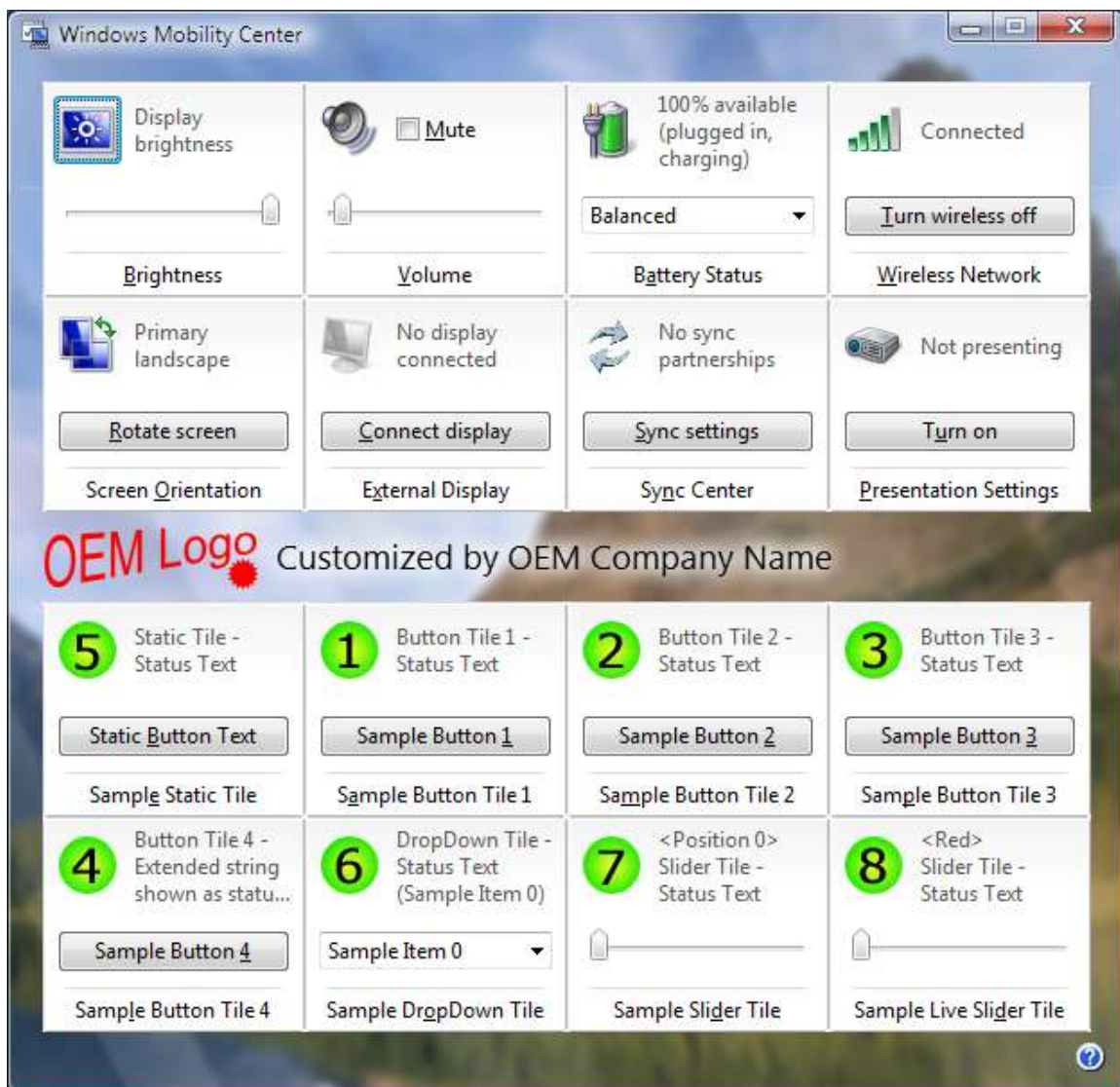
Figure 6: UI presented by Windows Mobility Center that shows 1 static tile and 7 dynamic tiles. Only tiles listed in the TileOrder value will be shown in Windows Mobility Center. Any of the sample tiles can be removed from the UI by removing its name from the TileOrder registry value.
